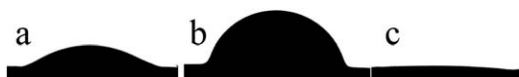
Figure 2. Contact angle measurements of the (a) pristine PVA-co-PE nanofiber membrane, (b) BIBB-activated PVA-co-PE nanofiber membrane, and (c) PSBMA-functionalized PVA-co-PE nanofiber membrane.
